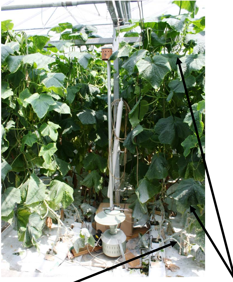
Figure 7. Burkard (large light green unit at base of crop) and MTIST (two small cylindrical units in upper & lower parts of the crop canopy) air samplers in position at Anchor Nurseries
